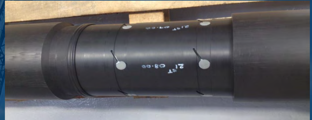
Modified LinerBridge ® internal energisation system under testing
