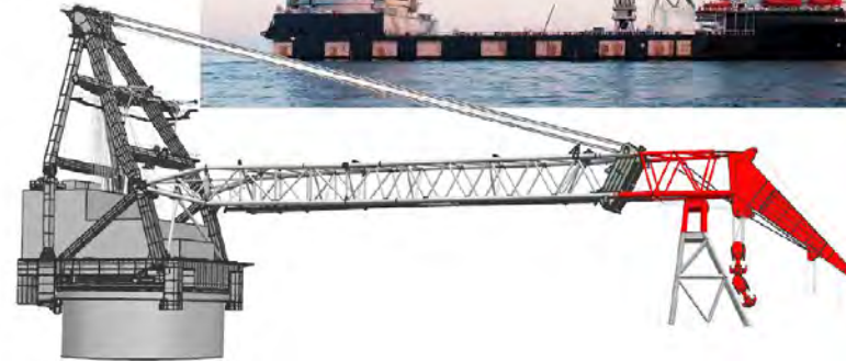
Q3 – 2020 Crane Upgrade Boom Extension
