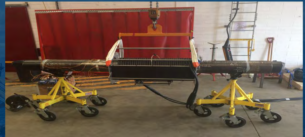
InsuLine ™ Sleeves under testing at 250 degC
